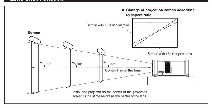
The separately sold lenses used on the projector have a lens shift function. With the lens used, you can adjust the projected image vertically using the setting menu or the remote control's SHIFT button U or D.
